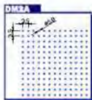
Hole size / Dia. 0.8mm Pitch: 3.0mm Open Area: 4.0%
