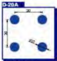
Hole size / Dia. 10.0mm Pitch: 30.0mm Open Area: 9%
