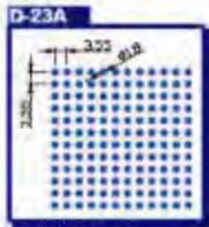
Hole size / Dia. 1.0mm Pitch: 3.0mm Open Area: 20%
