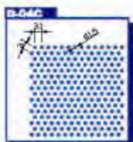
D-04C Hole size : Dia. 1.0mm Pitch : 2.0mm Open Area : 21.0%
