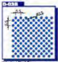
Hole size / Dia. 2.5mm Pitch: 5.0mm Open Area: 27.0%
