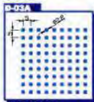
Hole size / Dia. 2.0mm Pitch: 5.0mm Open Area: 16.0%
