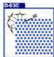
D-03C Hole size : Dia. 2.0mm Pitch : 4.0mm Open Area : 23%
