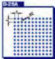
Hole size / Dia. 2.0mm Pitch: 4.0mm Open Area: 20%
